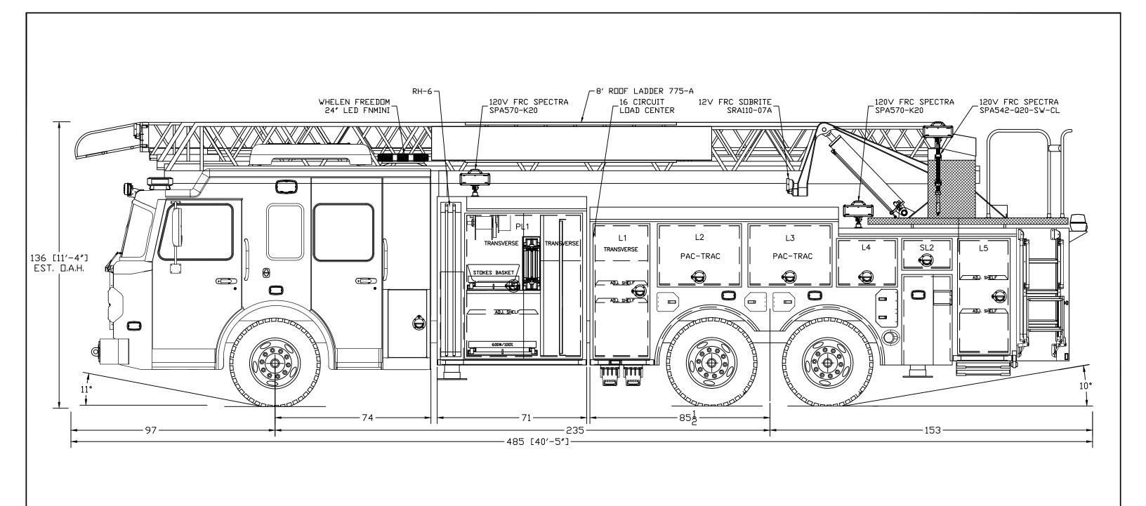
CHASSIS: GLADIATOR ELFD 10" RAISED ROOF WITH 10" NOTCH & DROP CAB GENERATOR: ONAN 10kW 10RBAB COMPARTMENTS: 425 CUBIC FEET ADDITIONAL PENETRATION STABILIZERS 304 STAINLESS BODY AND PUMP MODULE AL-11 AERIAL INFORMATION SYSTEM ON SCENE COMPARTMENT LIGHTING
