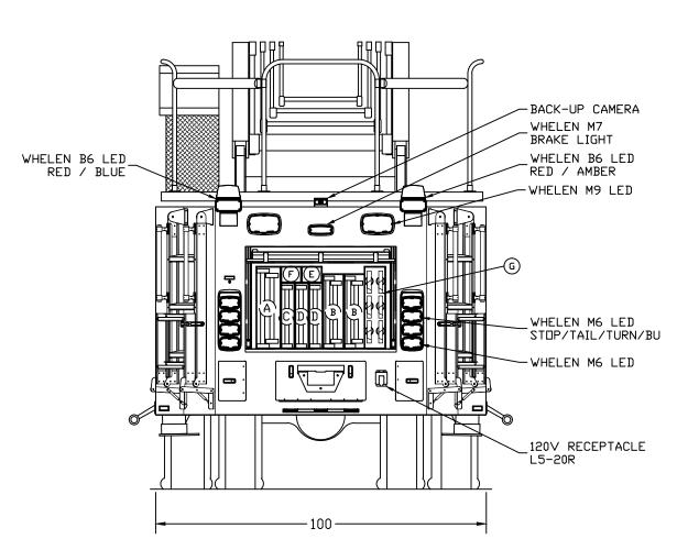
CHASSIS: GLADIATOR ELFD 10" RAISED ROOF WITH 10" NOTCH & DROP CAB GENERATOR: ONAN 10kW 10RBAB COMPARTMENTS: 425 CUBIC FEET ADDITIONAL PENETRATION STABILIZERS 304 STAINLESS BODY AND PUMP MODULE AL-11 AERIAL INFORMATION SYSTEM ON SCENE COMPARTMENT LIGHTING
