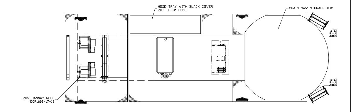
CHASSIS: GLADIATOR ELFD 10" RAISED ROOF WITH 10" NOTCH & DROP CAB GENERATOR: ONAN 10kW 10RBAB COMPARTMENTS: 425 CUBIC FEET ADDITIONAL PENETRATION STABILIZERS 304 STAINLESS BODY AND PUMP MODULE AL-11 AERIAL INFORMATION SYSTEM ON SCENE COMPARTMENT LIGHTING
