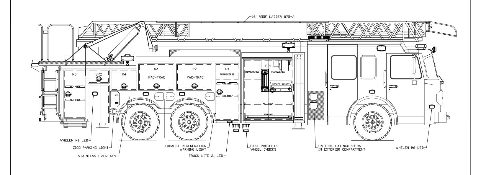
CHASSIS: GLADIATOR ELFD 10" RAISED ROOF WITH 10" NOTCH & DROP CAB GENERATOR: ONAN 10kW 10RBAB COMPARTMENTS: 425 CUBIC FEET ADDITIONAL PENETRATION STABILIZERS 304 STAINLESS BODY AND PUMP MODULE AL-11 AERIAL INFORMATION SYSTEM ON SCENE COMPARTMENT LIGHTING
